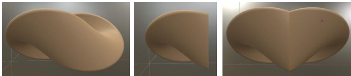
Figure 6.5 Views of the slice and mirror process in 3D Coat
