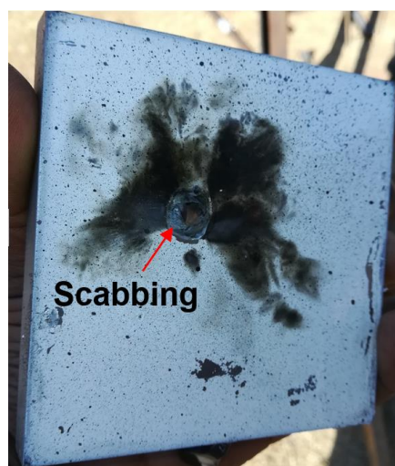
Figure 4.4: Scabbing a 14 mm thick plate
