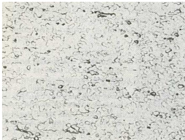
Figure 2.10: Ti6Al4V primary alpha ( \alpha_p ) phase and small amounts of untransformed \beta -phase after solution heat treatment at 843°C and then water quenching [28]
