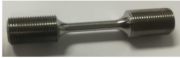
Figure 3.2: Machined wrought Ti6Al4V tensile sample
