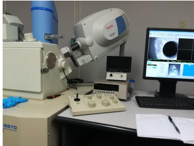
Figure 3.10: The JEOL JSM-6610 scanning electron microscope used in this study
