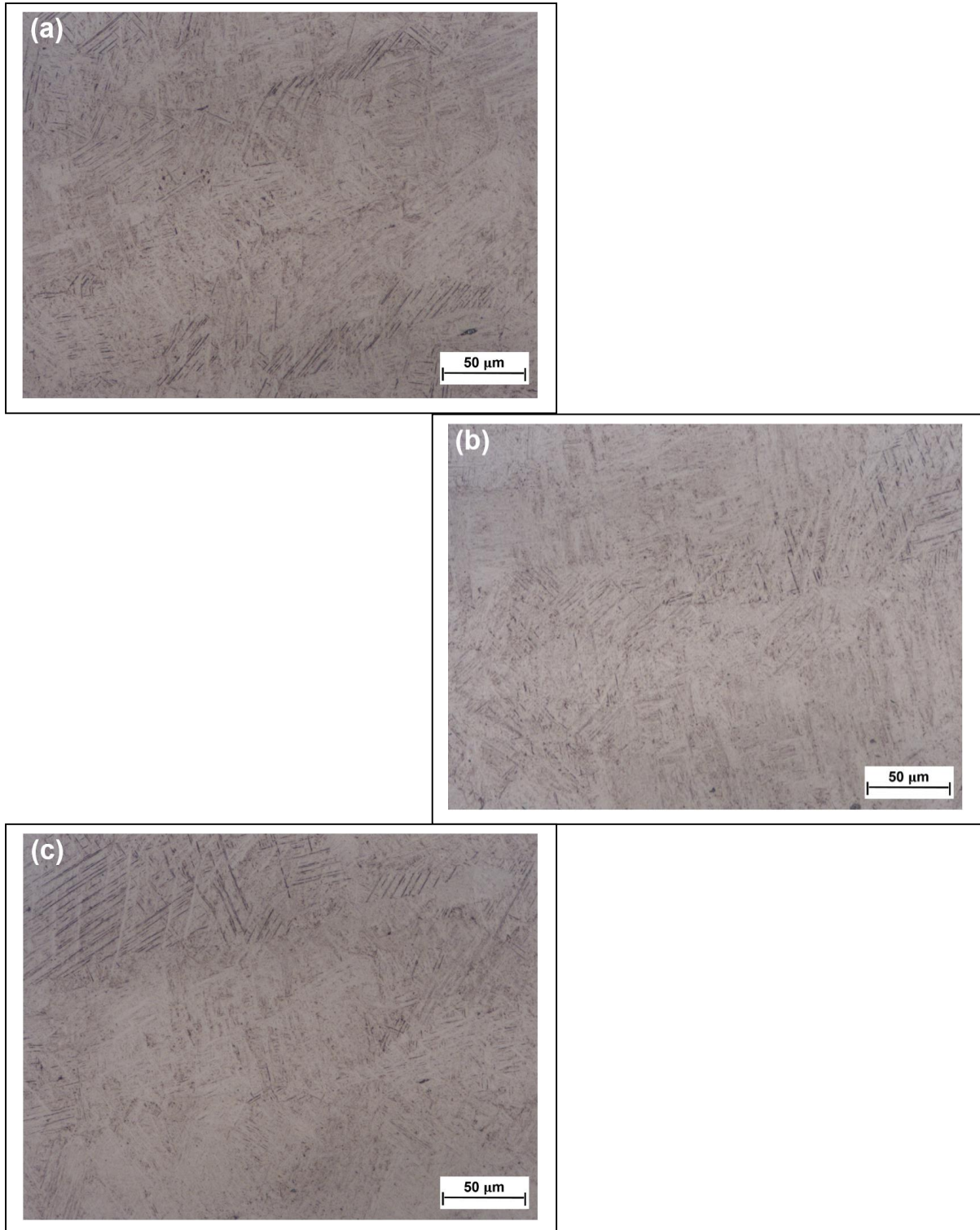
Figure 4.79: Optical micrographs at a distance of 4 mm from the edge of the projectile holes through the 8 mm thick plates
