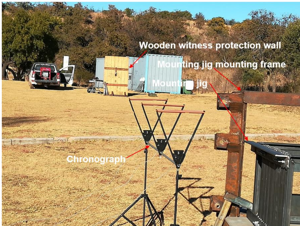
Figure 3.5: Image of the test setup on the Gerotek testing range
