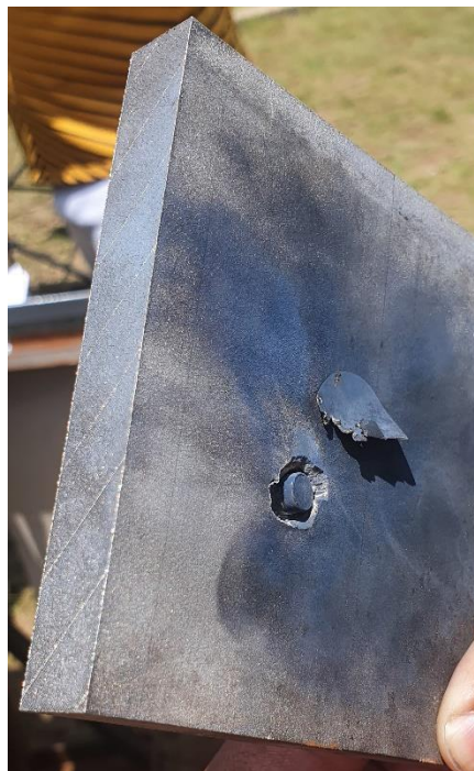
Fail: Full Penetration
