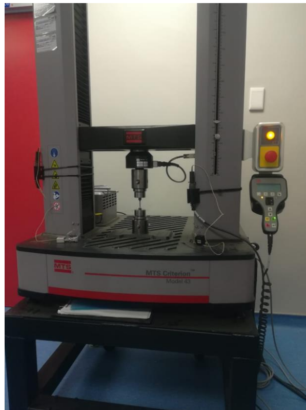
Figure 3.4: MTS Criterion model 43 tensile testing machine and test set up
