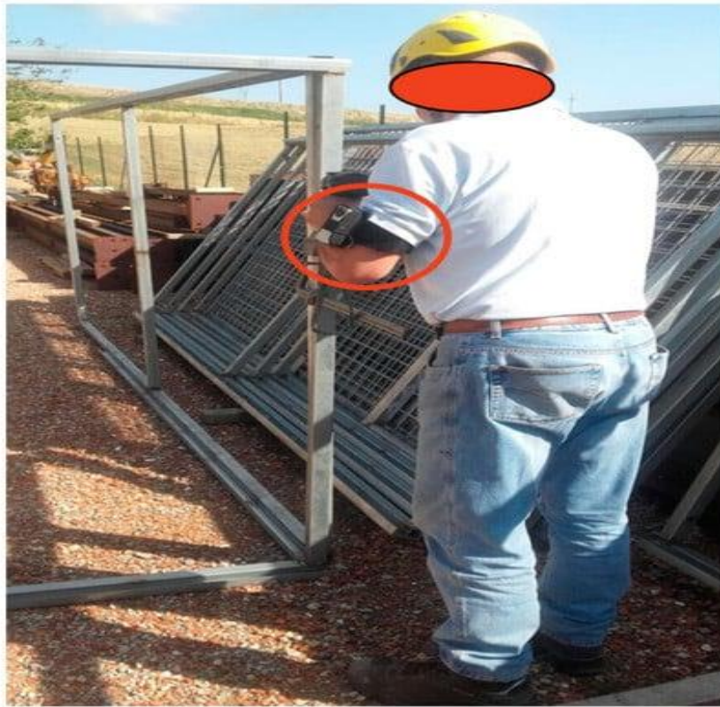
Figure 3.6: A construction worker wearing the GENESIS-UV dosimeter on the upper left arm (Modenese et al., 2020)
