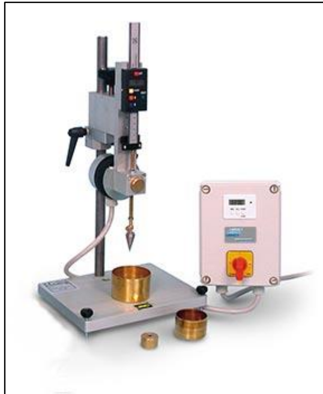
Figure 2-6: Typical BS fall-cone apparatus (BS 1377-2, 1990)
