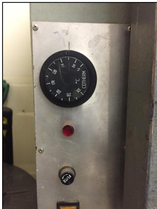
Figure 3-2: Oven used with temperature set to 45°C
