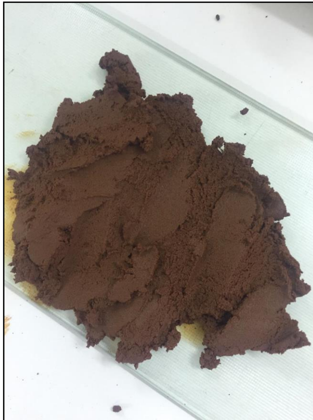
Figure 3-8: Soil after at least 16 hours of absorption and with sufficient moisture content to start the fall-cone test
