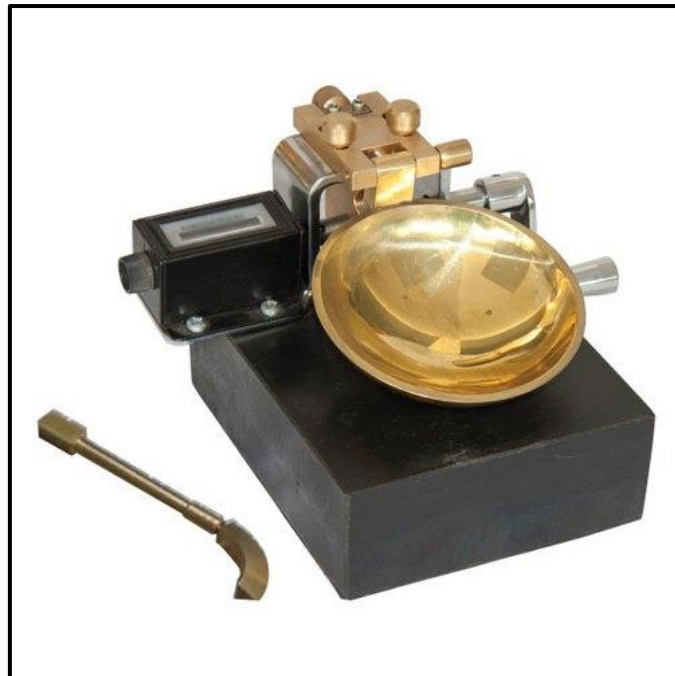
Figure 2-3: Typical Casagrande cup apparatus
