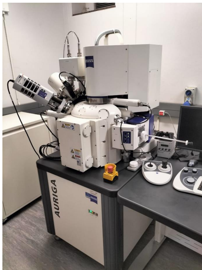
Figure 3.2 A scanning electron microscope (ZEISS-Auriga Cobra, Germany) used for observing the surface morphology of the samples.
