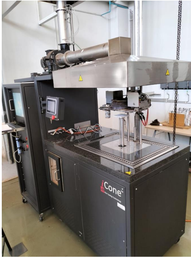
Figure 3.6 A cone calorimeter used for investigating the flammability properties of the samples.
