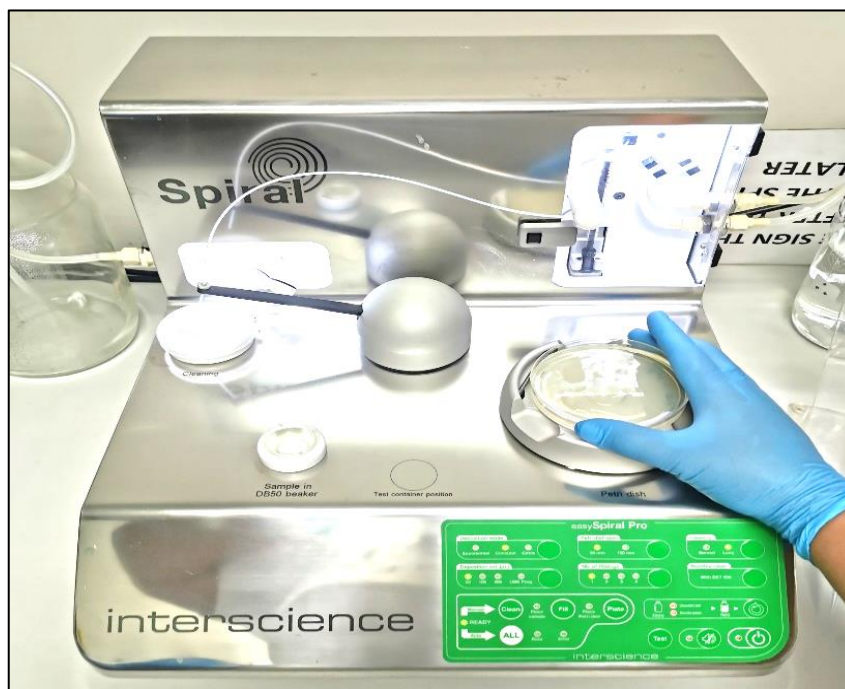
Figure 3.5: EasySpiral Pro® automatic plater (interscience). The easySpiral Pro® patented technology allows the automatic plating of samples on a Petri dish in only 25 seconds.
