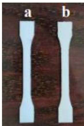
Figure 3.5: Image of tensile specimens of the (a) neat PLC and (b) 97/3 w/w PCL/EA nanocellulose composite
