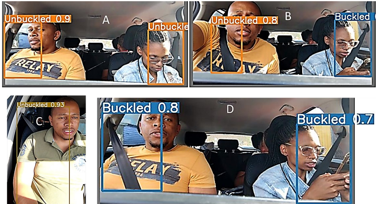
Fig 4.6: A, B, C, and D depict the safety belt detection status when the model was tested in occluded and visible pillar loop conditions.
