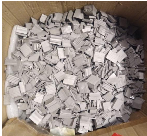
Figure 3-18. Ti6Al4V(ELI) scrap resulting from removing supports of DMLS-produced hierarchical HC parts
