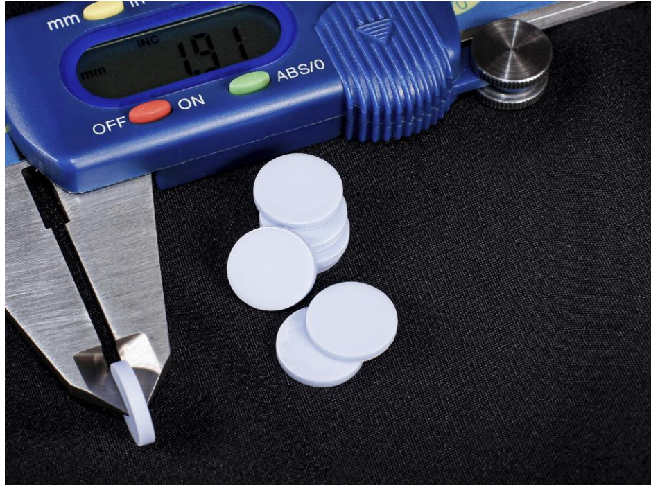
Figure 3-7: HA480 non-porous disc scaffold for cell culture.
