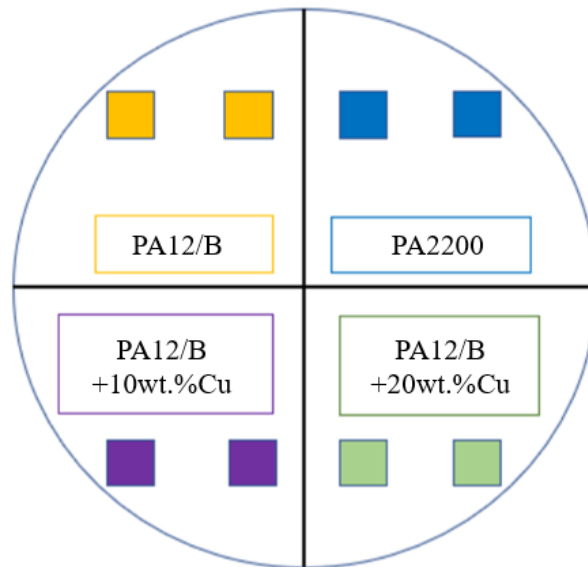
Figure 39. Schematic overview of sample distribution for performing the experiments on the antibacterial effect of ion diffusion in Petri dishes
