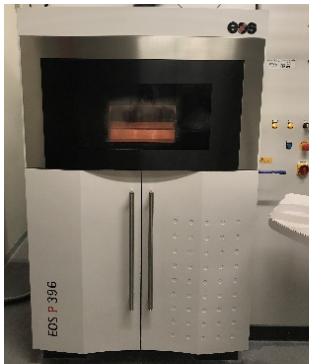
Figure 30. EOSINT P396 SLS 3D printer machine installed at CRPM, CUT
