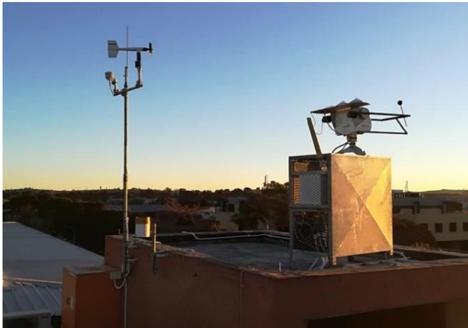
Figure 4.1: Irradiance, temperature and wind sensors located at CUT [49]
