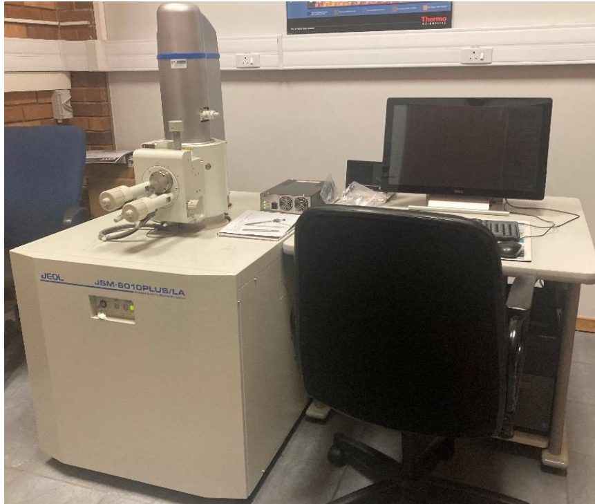
Figure 3.8: JOEL JSM-6010Plus/LAM scanning electron microscope.
