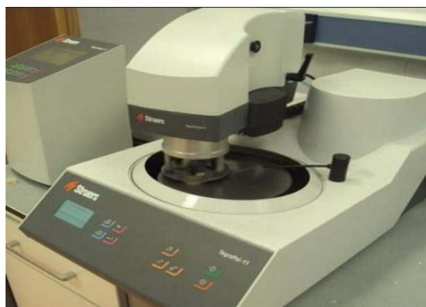
Figure 3.17: Struers TegraPol31 automatic grinding and polishing machine.
