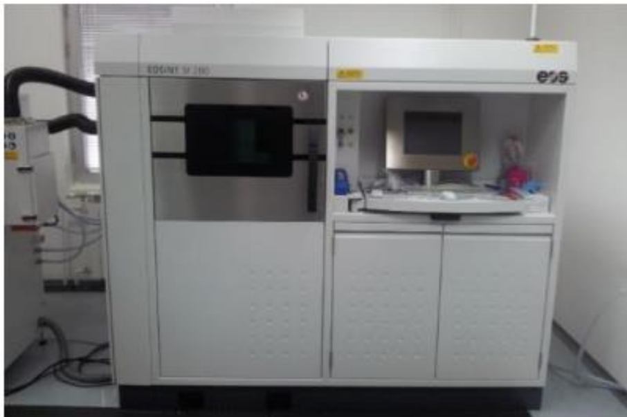
Figure 3.7: EOS M280 machine used.
