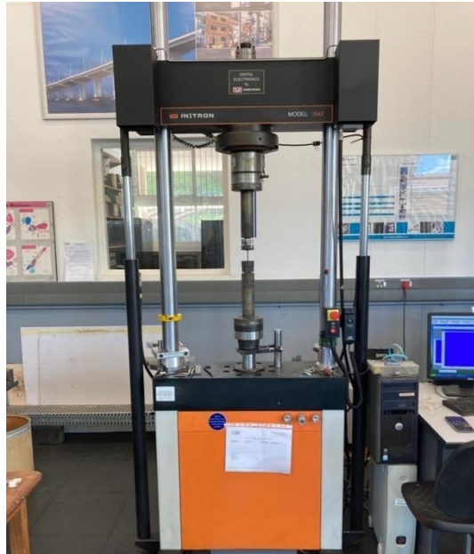
Figure 3.13: Instron 1342 mechanical testing machine used in this study.
