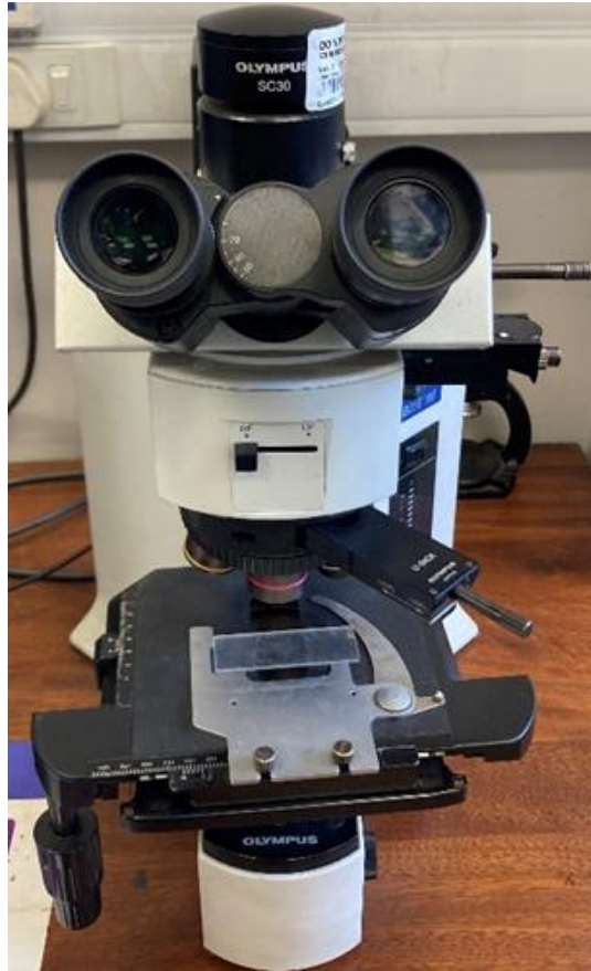
Figure 3.9: Olympus BX51M optical microscope.
