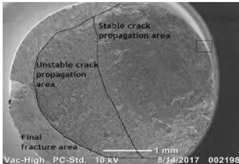
Figure 2.28: Fracture surface showing different stages of crack propagation [153].
