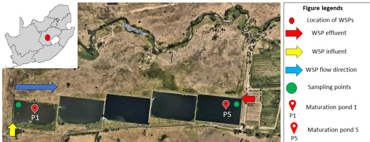
Figure 3.1: The location and the configuration of the maturation ponds in Bloemspuit, South Africa.
