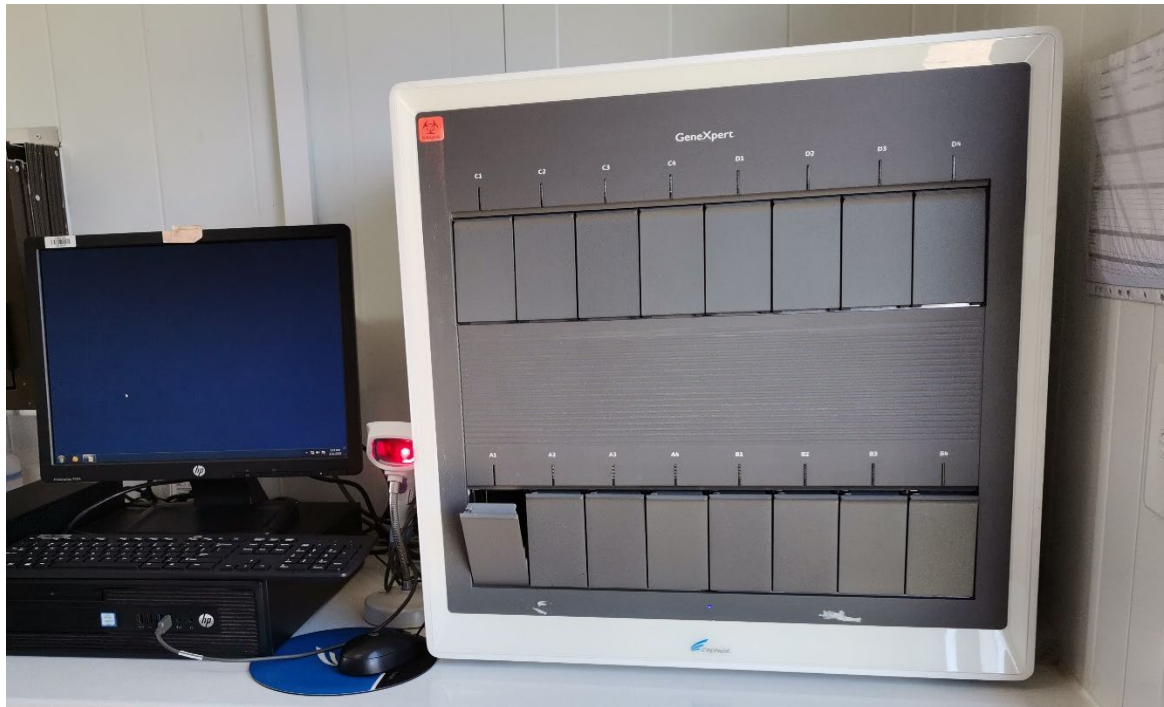
Figure 2.8: GeneXpert XVI, which is a version that has 16 modules and a desktop computer
