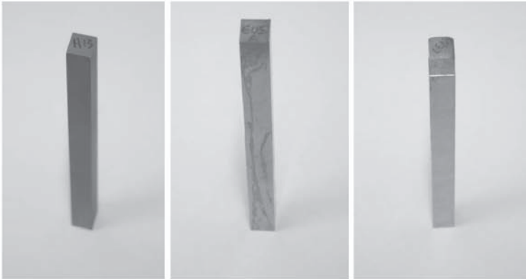
Figure 2: Pictures showing the cores manufactured with the conventional and RP methods. From left to right: Through-hardened steel H13 conventional manufactured specimen, EOS-DMLS grown specimen, LENS grown specimen
