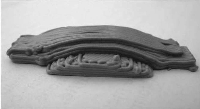
Figure 10: First complete curved-layer part produced by modified Fab@home rapid prototyping machine
