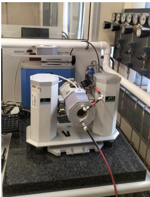
Figure 3.8: Perkin-Elmer DMA used to determine mechanical properties
