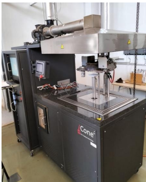
Figure 3.6: Cone calorimeter used for the analysis of the flammability of samples
