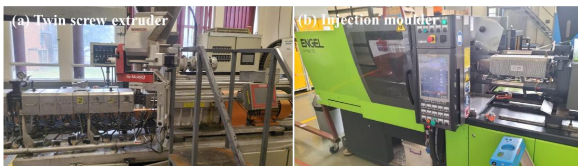
Figure 3.3: Machines used for (a) compounding and (b) moulding test specimens
