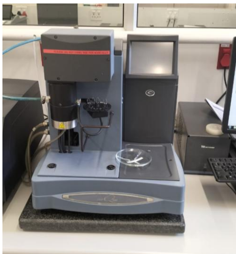
Figure 3.5: Thermogravimetric analyser used to analyse thermal stability
