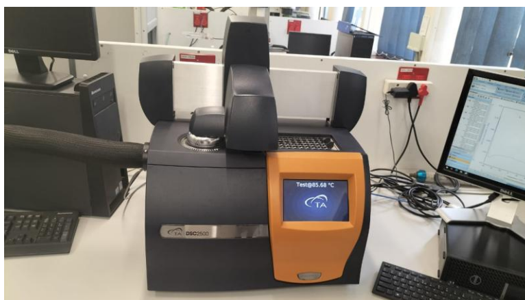
Figure 3.11: DSC machine used to measure the heat transfer of samples
