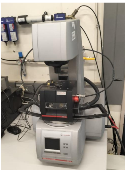
Figure 3.7: Equipment that was used to determine the dynamic rheological measurements
