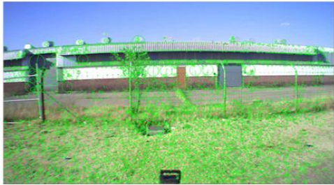
Figure 5. Detecting the image feature using SIFT algorithm
