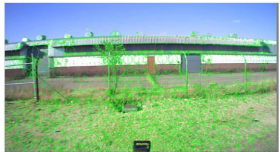
Figure 6: Detecting the image feature using SIFT
