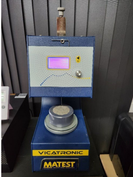
Figure 3.7: Vicatronic automatic recording apparatus (Vicat)
