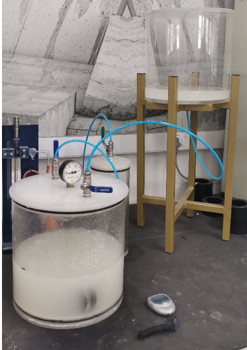
Figure 3.12: Water sorptivity index samples in a vacuum tank filled with calcium hydroxide solution
