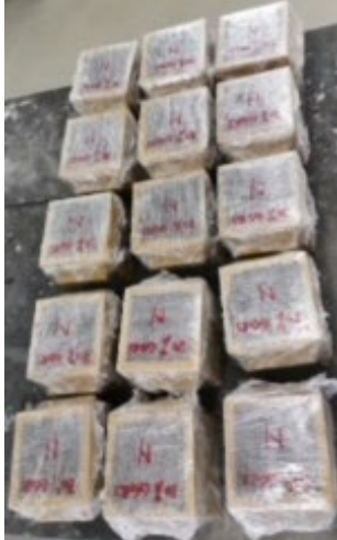
Figure 3.9: 100 x 100 ambient-cured GPC samples
