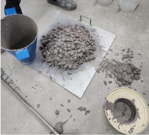
Figure 3.6: Concrete slump test equipment
