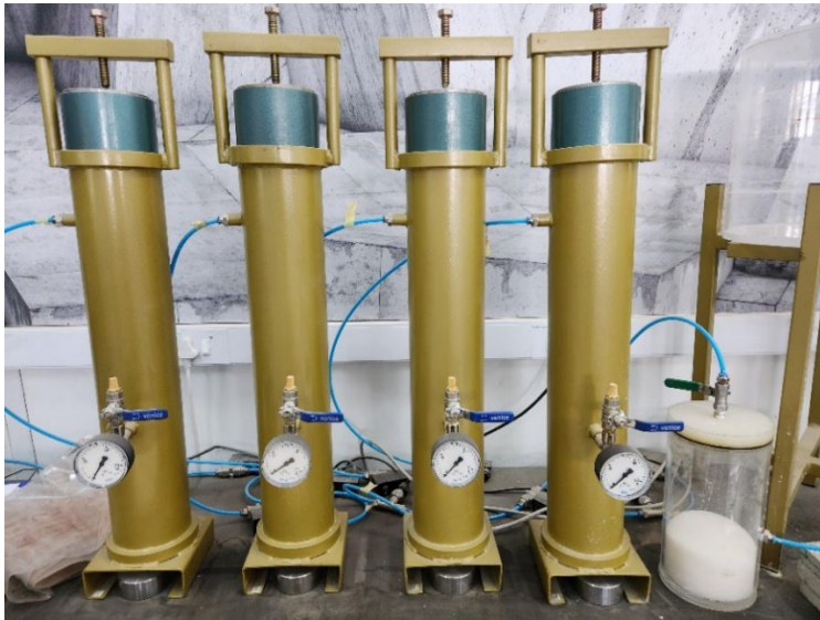
Figure 3.11: Permeability cells for oxygen permeability index testing
