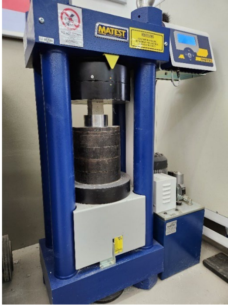
Figure 3.8: Automatic Max testing machine for compressive strength test
