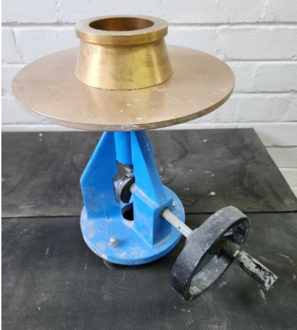
Figure 3.5: Flow table apparatus
