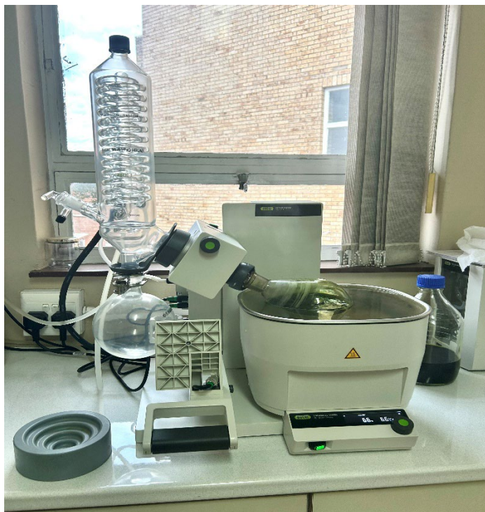
Figure 4.3: The rotary evaporator used for concentrating the extracts
