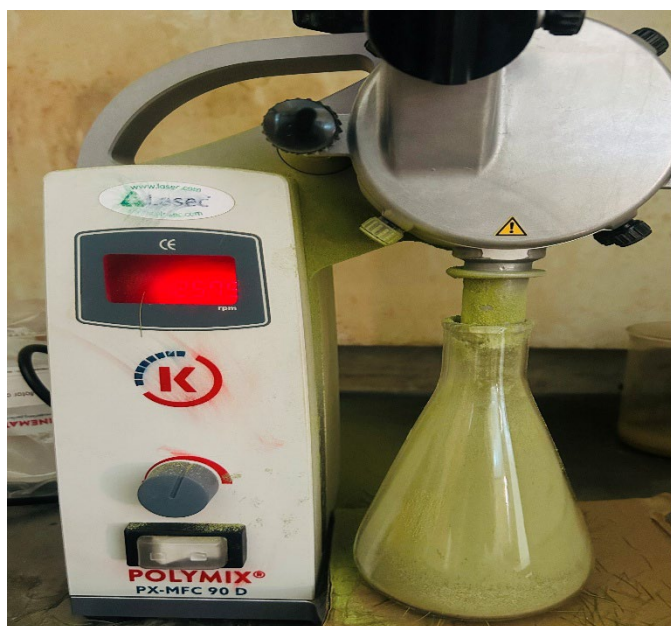
Figure 4.2: The grinding machine used to grind Asparagus Laricinus plant leaves
