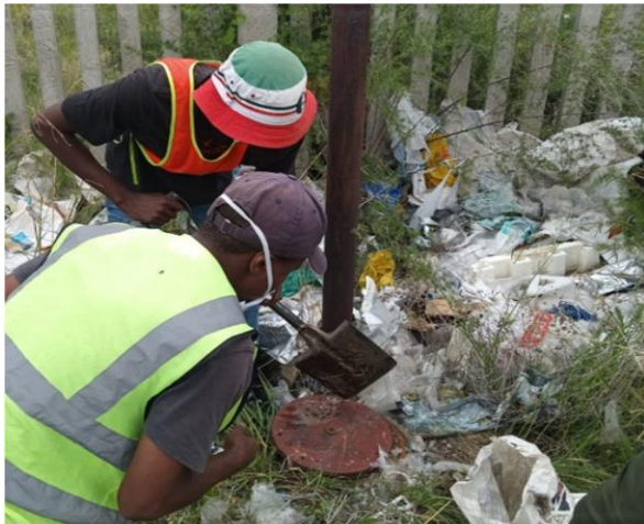
C – Borehole inside the landfill on the margin of the landfill located close to a pole for easy identification
