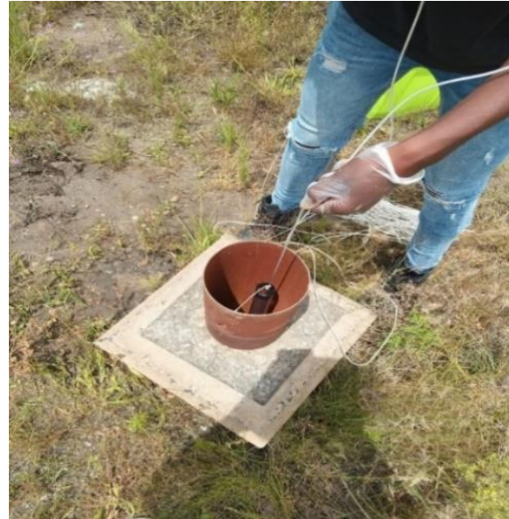
B – The bailer is inserted into the borehole for rinsing three times repeatedly
