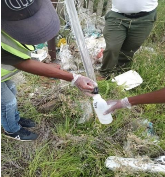
A – Filling the plastic bottle with groundwater using bailer for physicochemical parameters
