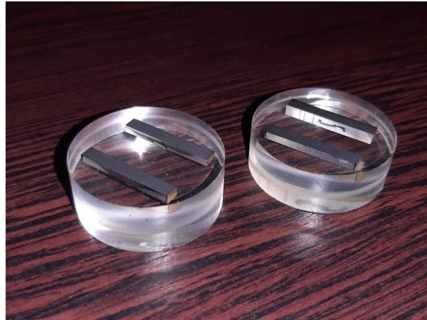
Figure 16: Polished specimens of single-track builds without powder after mounting, polishing, and etching
