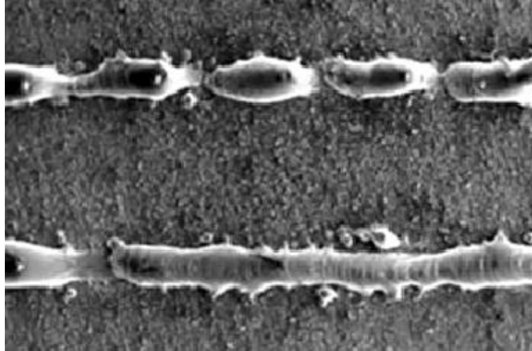
Figure 4: Incidences of balling of the melt pool due to too high scanning speeds (Li et al., 2011)
