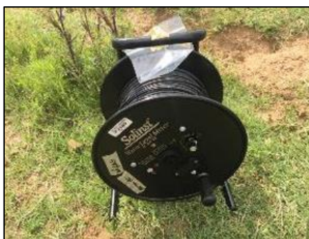
Figure 4.13 Solinst meter used for calculating groundwater level (Author, 2023)
