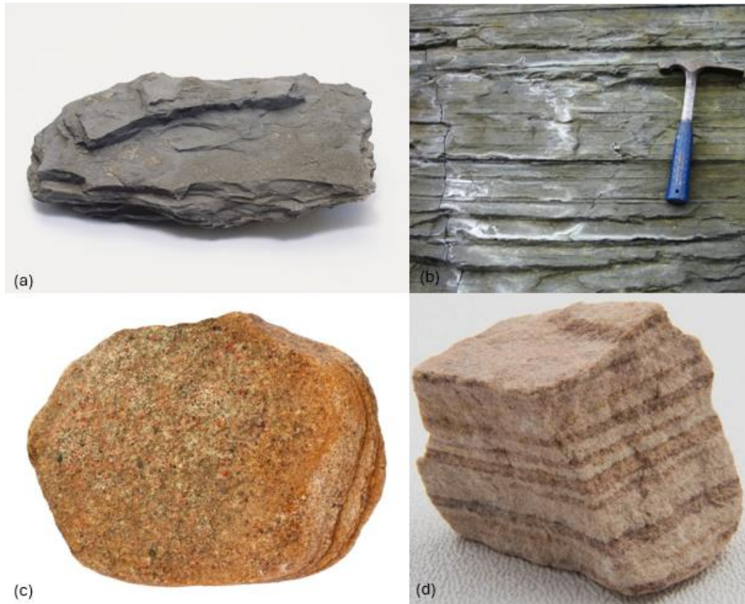
Figure 3.11 Images showing (a) shale stone, (b) layered shale stone formation, (c) sandstone and (d) layered sandstone formations (Author, 2024)
