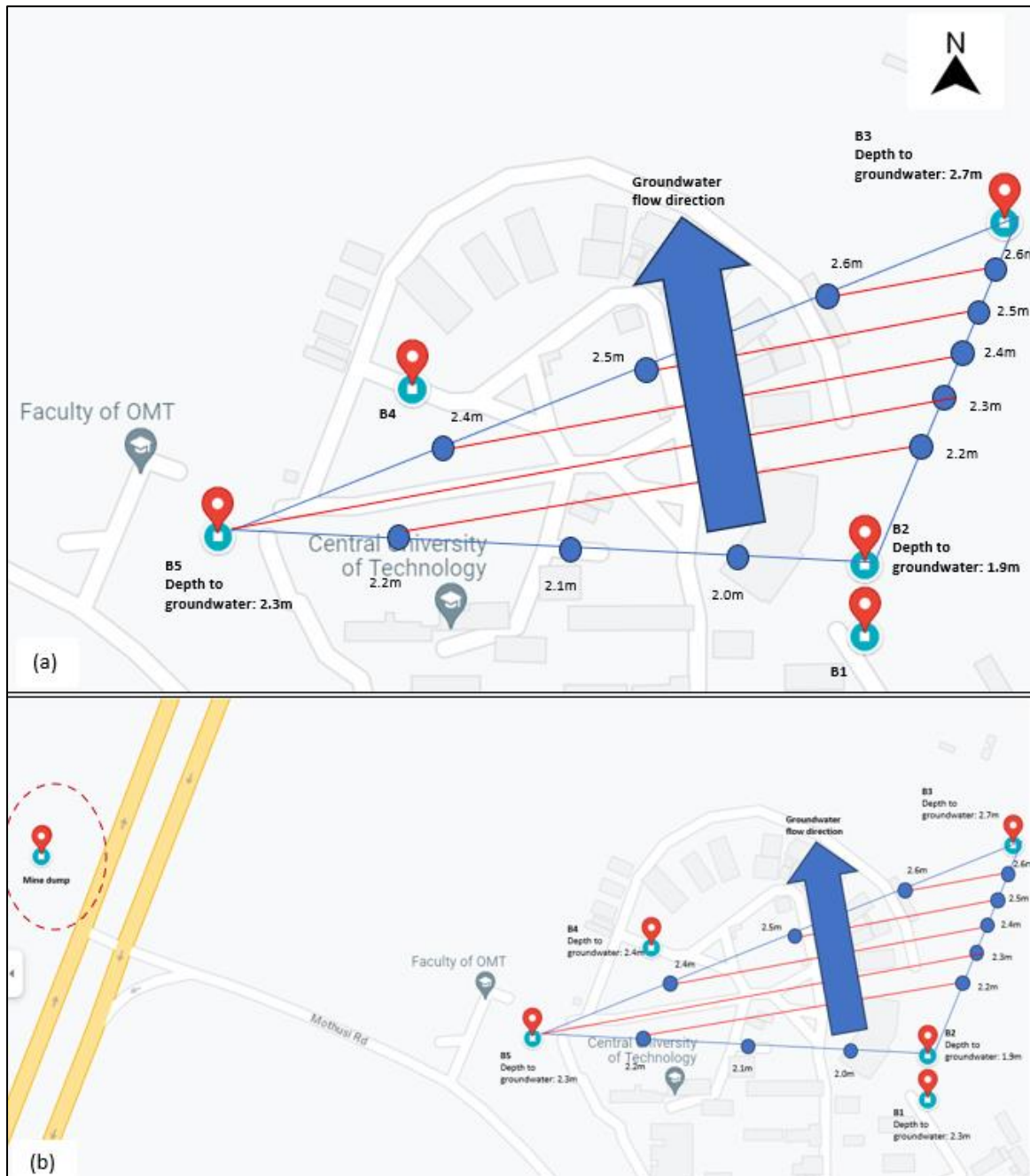
Figure 4.17 (a) Proposed groundwater flow direction across the five boreholes, (b) Groundwater flow direction relative to the mine dump (Google Maps, 2023)
