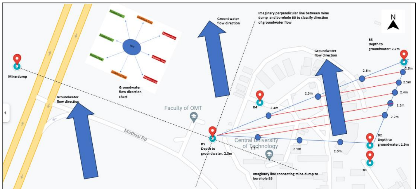
Figure 6.6 Groundwater flow direction relative to the groundwater flow chart and the mine dump
