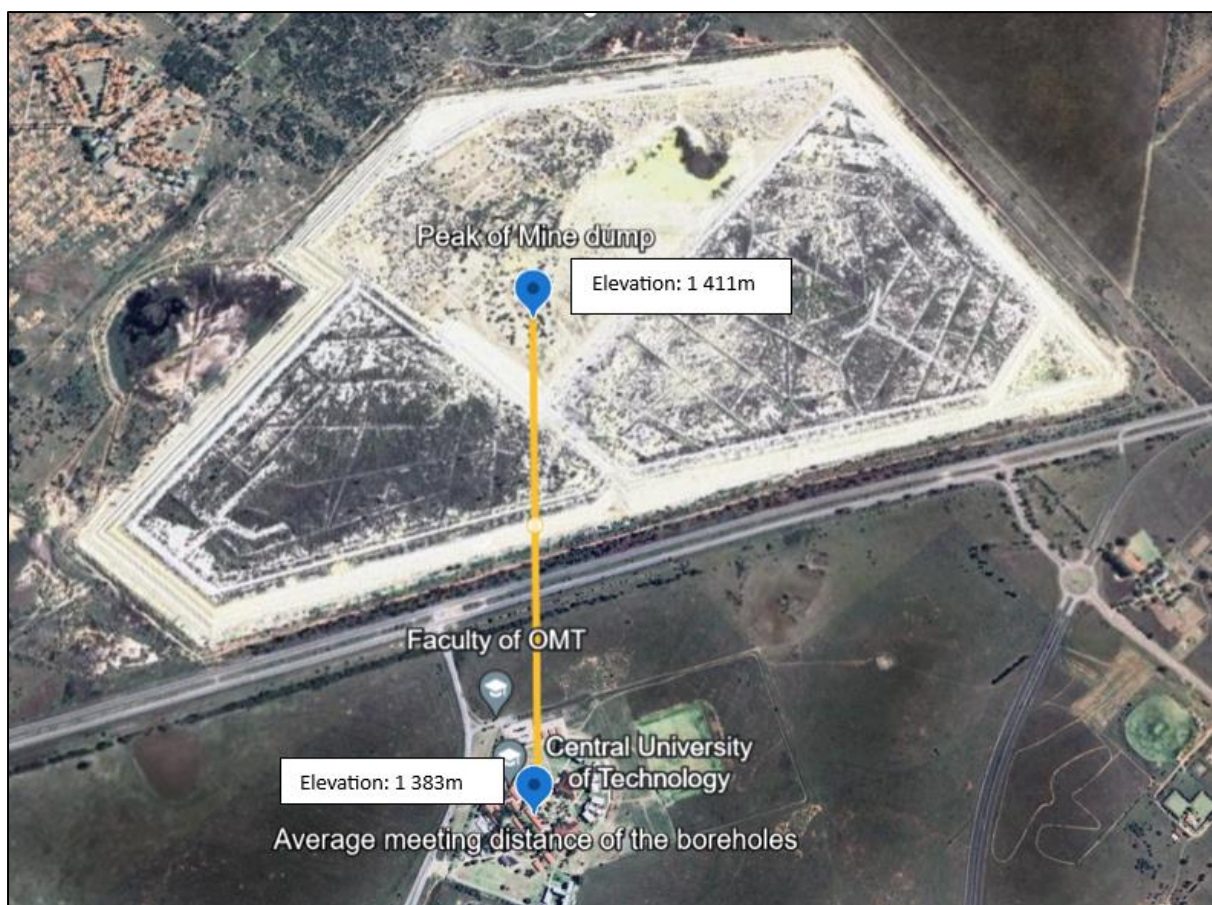
Figure 7.4 Elevation of the mine dump slope relative to the CUT Welkom campus boreholes
