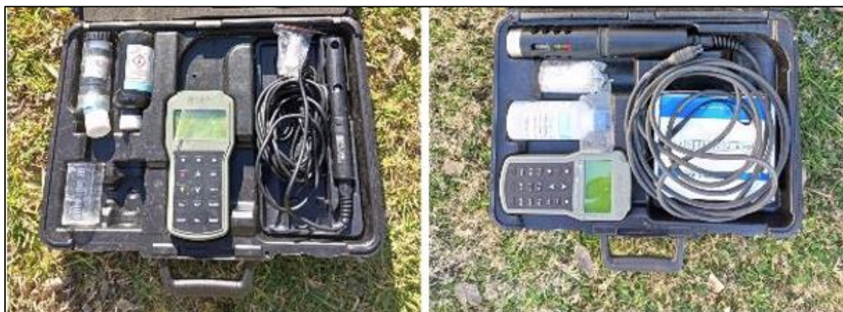
Figure 4.2 HANNA multiparameter waterproof meter set (HI98195) used to measure physical parameters and dissolved oxygen (Author, 2023)
