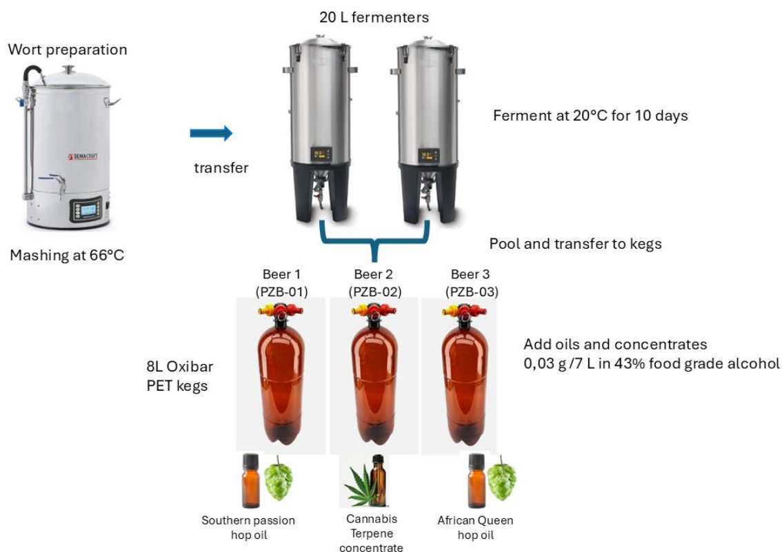
Figure 4.1: Diagram showing the brewing process, packaging and hop oil and cannabis terpene extract additions.
