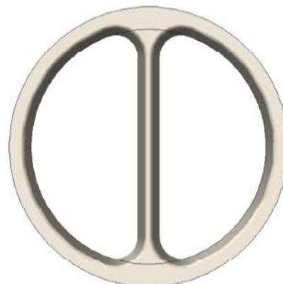
Figure 15: Circular section manufactured in a horizontal position with support.
