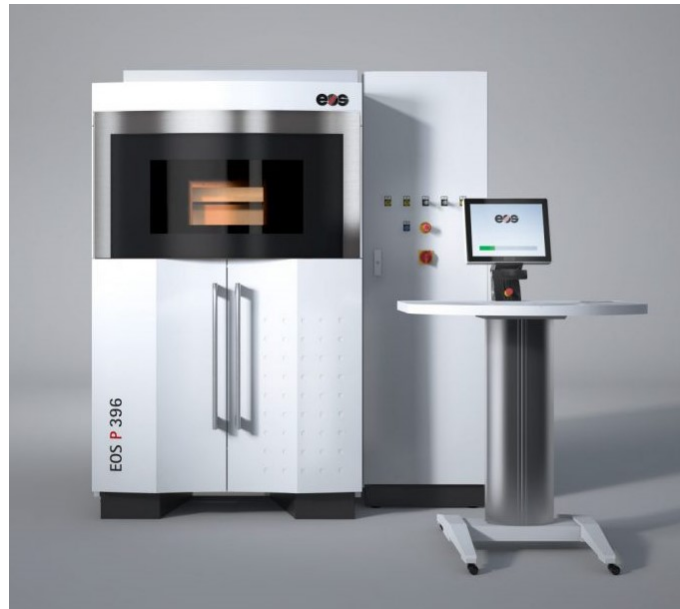
Figure 12: EOSINT P 396 SLS system (EOS SLS, 2021).
