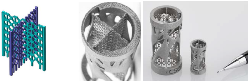
Figure 6. An interlocking flexure monolithic structure (Keiner et al., 2019).
