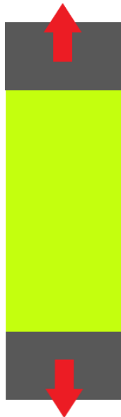
Figure 15: Scaffolding tensile test schematic. The green section shows the scaffolding area, the grey areas are solid and used to fasten the scaffolding in the machine, and the arrows indicate the directions in which the specimens were pulled.
