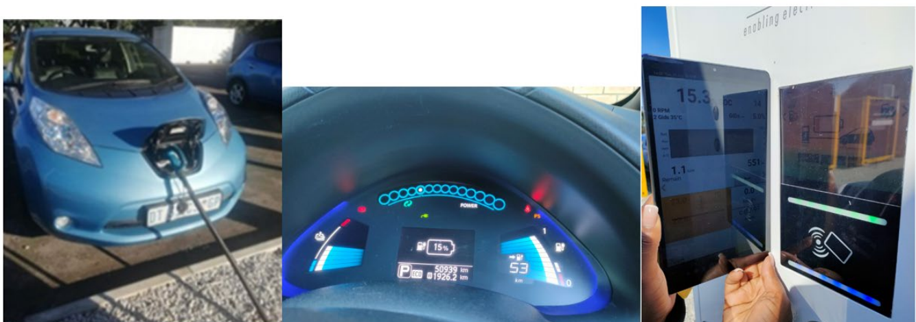
Figure 3.5: Minimum battery SoC for fast DC charging
