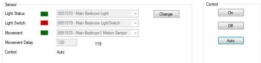
Figure 3.13 Controller's view: Movement sensor activates a light
