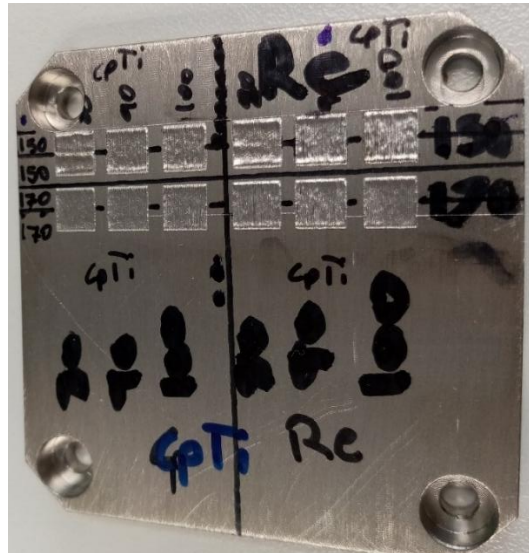
Figure 3.34: Double layers sintered on Ti6Al4V substrate
