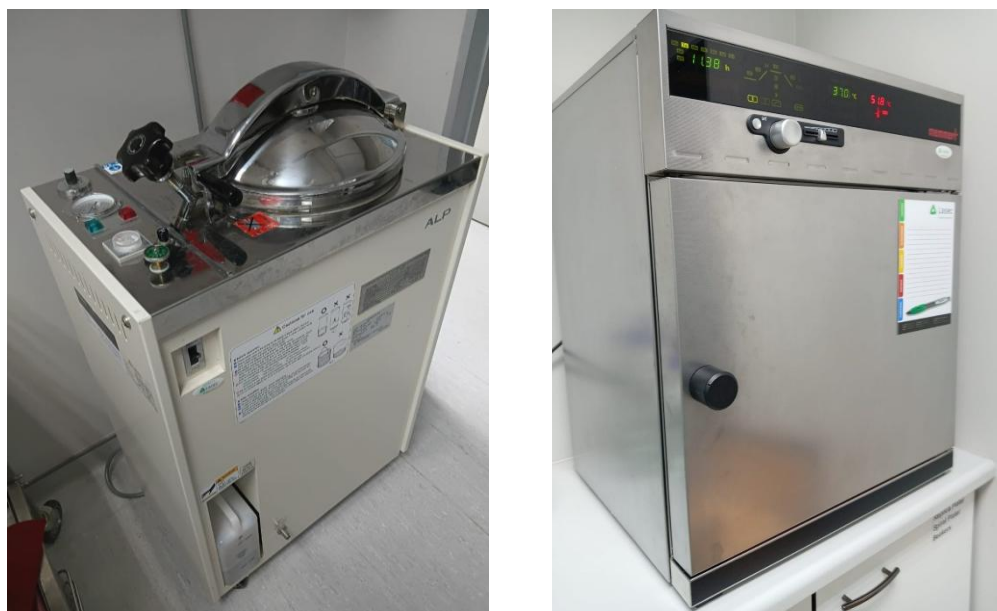
Figure 6.2: (i) ALP KT-30L Autoclave, and (ii) Precision Incubator Memmert INB
