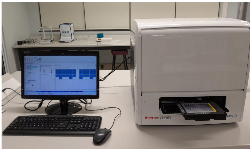
Figure 6.8: Varioskan LUX Multimode Microplate Reader
