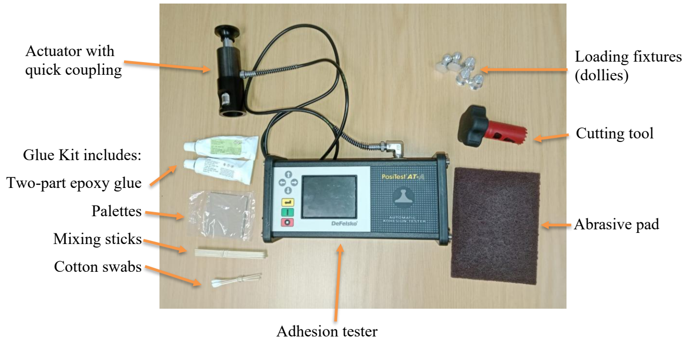
Figure 5.3: DeFelsko PosiTest AT-A automatic Adhesion Tester kit
