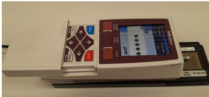
Figure 3.9: Mitutoyo SURFTEST SJ-210 profilometer
