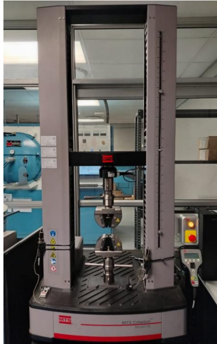
Figure 4.4: MTS Criterion Model 43 electromechanical universal testing machine
