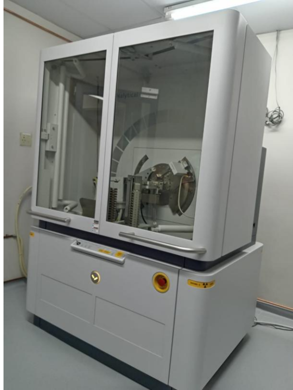
Figure 4.1: Malvern PANalytical Empyrean X-Ray diffractometer located at the University of the Free State
