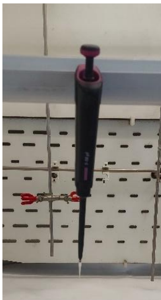
Figure 5.7: Micropipette setup for coating of metal substrates with polymer primer
