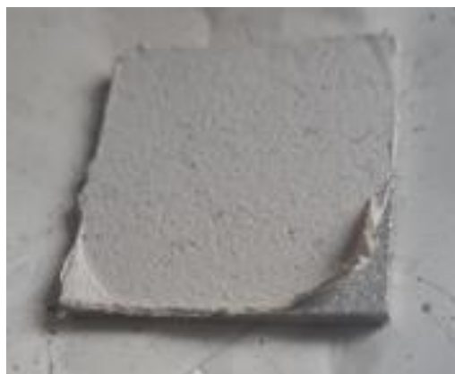
Figure 5.9: Electrospun PCL/PU/CuO (3:2:0.5, w/w/w) polymer NF mat peeling off from substrate
