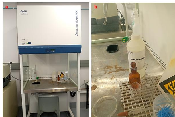
Figure 3.18 Equipment and material used for etching of specimens
