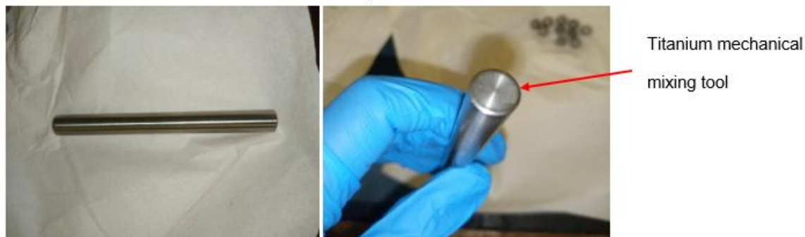
Figure 3.6 Images of a Ti6Al4V(ELI) tool used in manual mixing (a) length of tool, (b) diameter of tool
