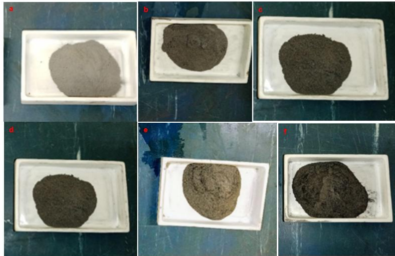
Figure 8.A Combined mixing powder samples at (a) 3 % vol. of CNTs, (b) 8 % vol. CNTs, (c) 15 % vol. CNTs, (d) 20 % CNTs, (e) 25 % CNTs, and (b) 30 % vol. of CNTs dispersed in a Ti6Al4V (ELI) matrix
