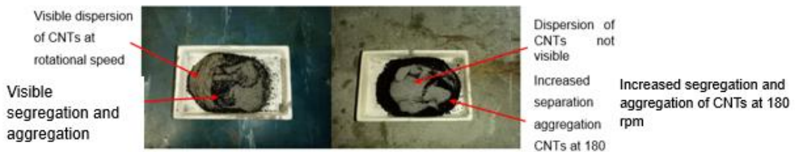
Figure A.6 Turbula mixed samples for 20 % vol. of CNTs dispersed in Ti6Al4V(ELI)
