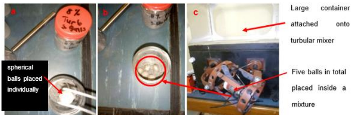
Figure 3.10 Steps carried out to mix powder samples using a turbula mixer
