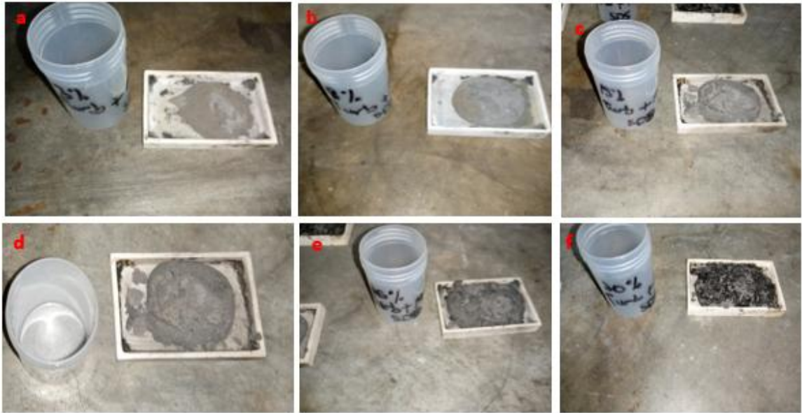
Figure A.13 Powder mixtures after oven-drying (a) 3 % vol. CNTs, (b) 8 % vol. CNTs, (c) 15 % vol. CNTs, (d) 20 % vol. CNTs, (e) 25 % vol. CNTs, and (f) 30 % vol. CNTs
