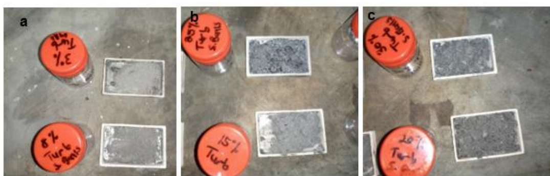
Figure A.12 Powder samples after oven-drying (a) 3 % and 8 % vol. CNTs/SDS powder samples, (b) 15% and 25% vol. CNTs/SDS powder samples, (c) 20 % and 30 % vol. CNTs/SDS powder samples
