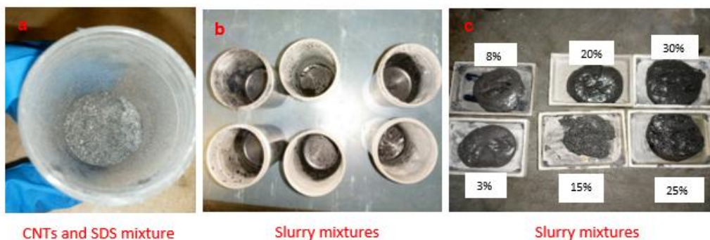
Figure A.9 Powder mixtures at various stages of mixing (a) mixture of CNTs and SDS, (b) slurry comprising CNTs, SDS, Ti6Al4V(ELI) and ethanol, (c) slurry placed on zircon plates for oven-drying
