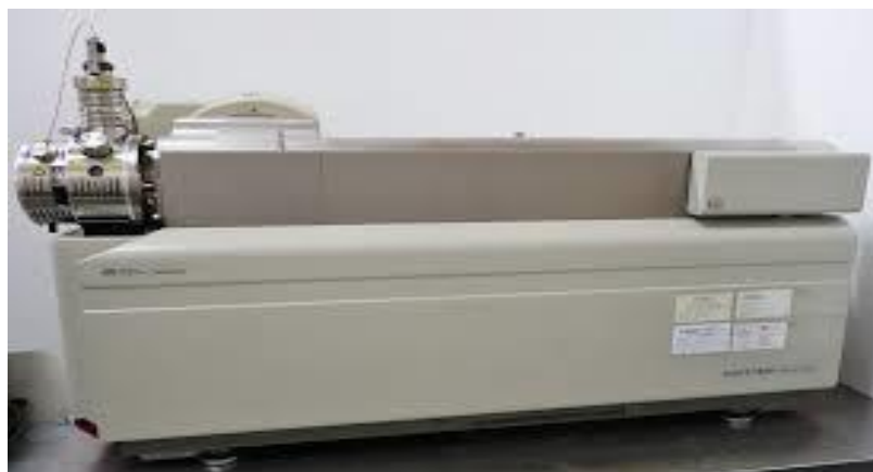
Figure 3.7 ABSCIEX 4000 QTRAP hybrid quadrupole ion trap mass spectrometer
