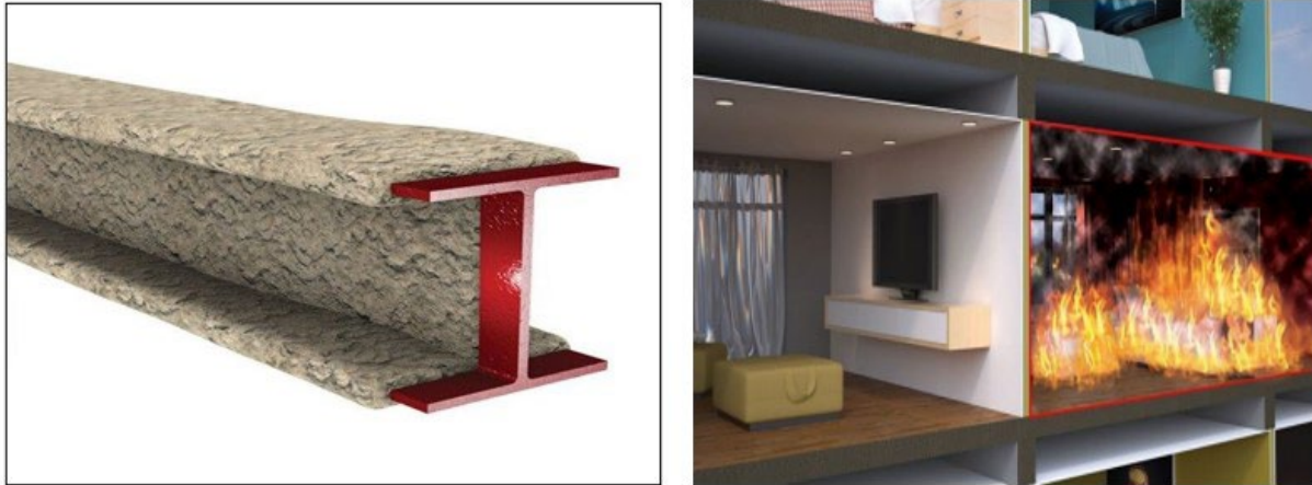
Figure 6. (a) Charred intumescent coating, (b) Fire boards as a measure of compartmentation
