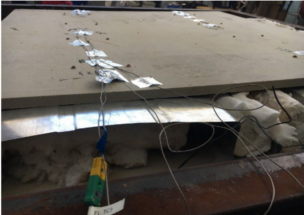
Figure 21. Side view of the prefabricated sandwich floor/ceiling system with a 20 mm thick FCB, placed on the furnace
