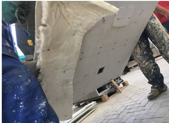
Figure 23. Broken sample with ceramic blanket patch, showing the exposed side
