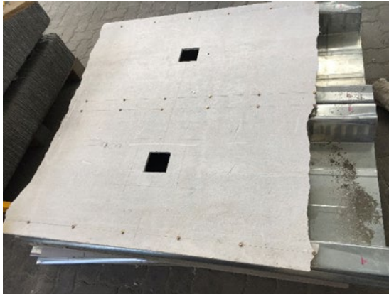
Figure 22. Broken sample, showing the exposed side
