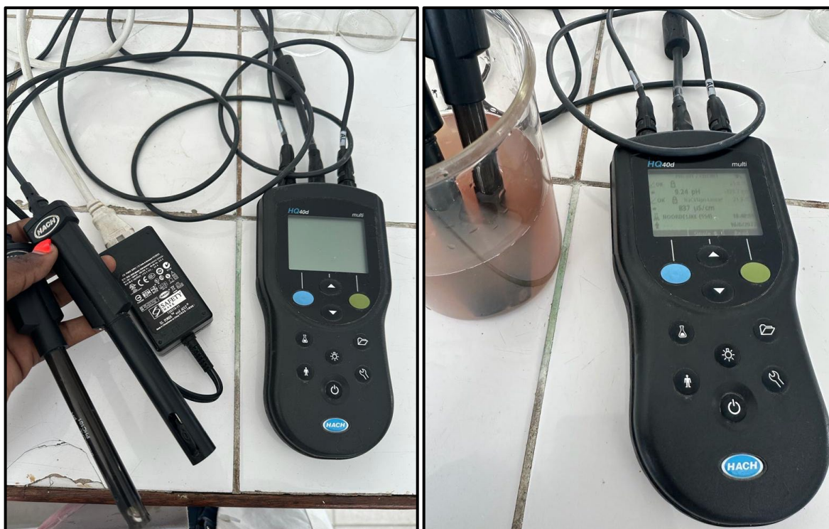
Figure 3.6: HQ40d probe for determining pH, conductivity, and temperature
