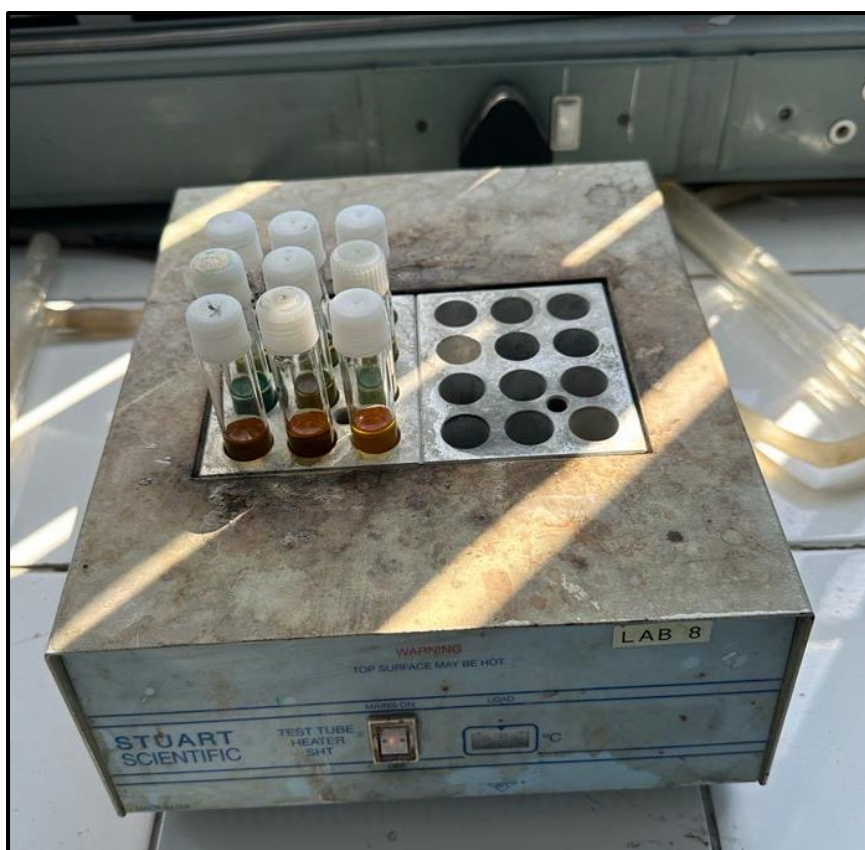
Figure 3.7: Example of the thermoreactor used to determine the COD
