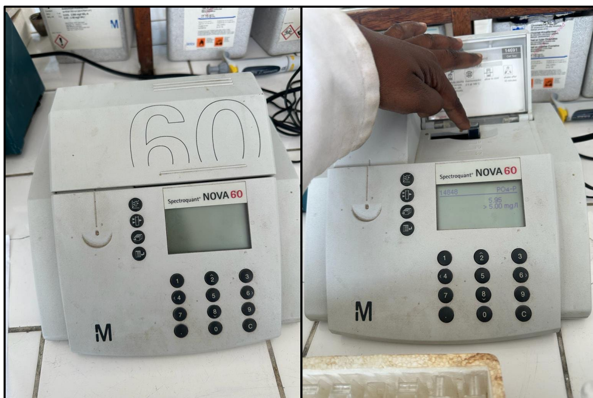
Figure 3.10: NOVA 60 Spectroquant® to determine the phosphate concentrations
