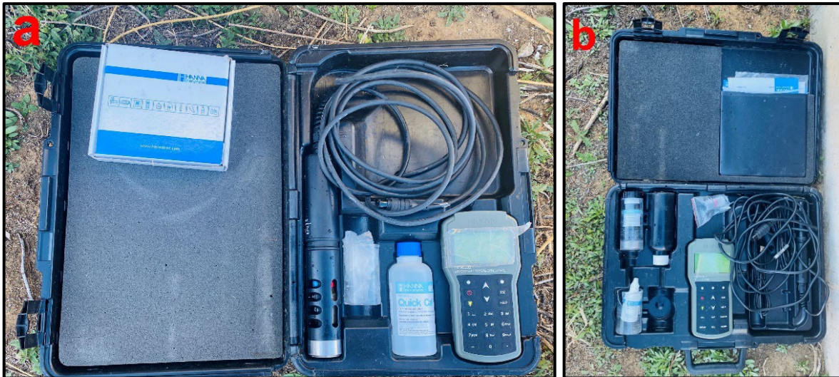
Figure 3.13: Example of HANNA probes used for the in-situ seasonal SW sampling: (a) HI 98195, and (b) HI 98193
