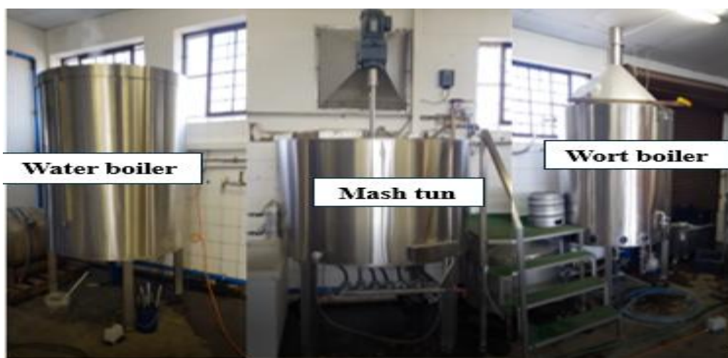
Figure 3.2: Key brewhouse equipment: Water boiler (left), mashing (mixer) (middle), and the wort boiler (right)
