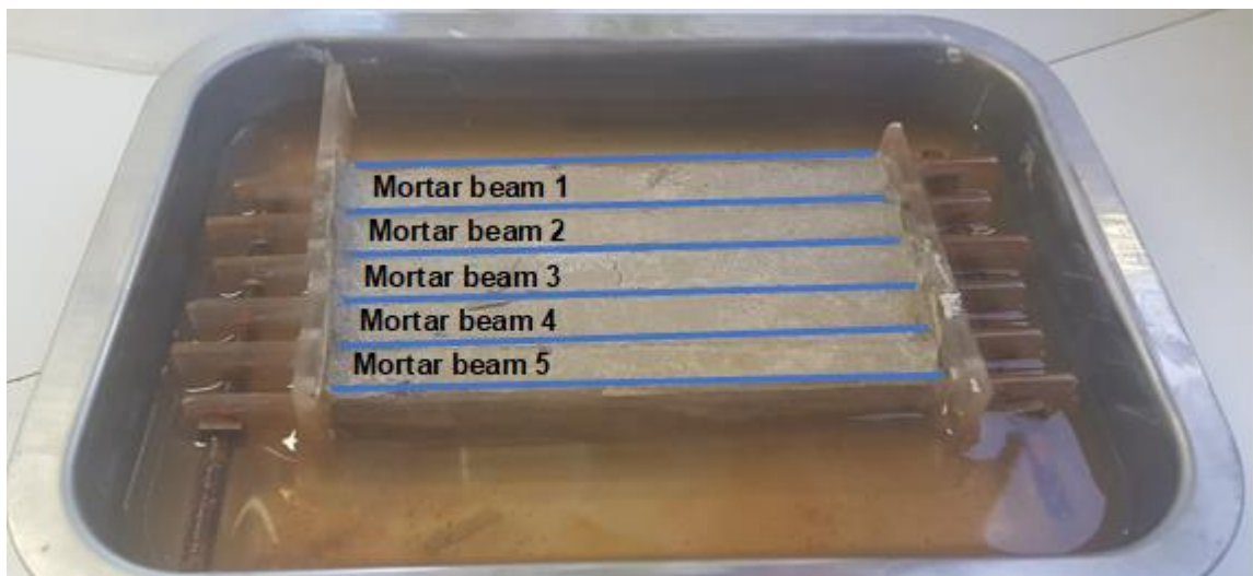
Figure 4.2: Five mortar beams in a mould
