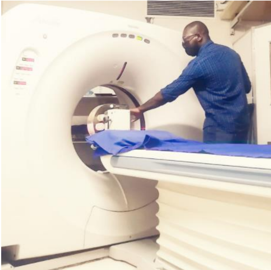
Figure 2.2: Test equipment being aligned (prepared for scanning) in the gantry aperture of a CT scanner.
