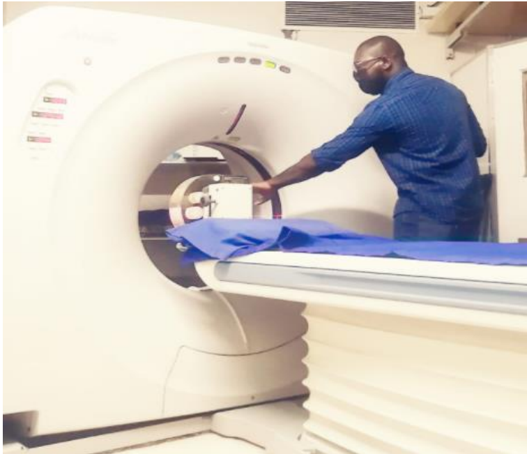
Figure 1. Test equipment being aligned (prepared for scanning) in the gantry aperture of a CT scanner.
