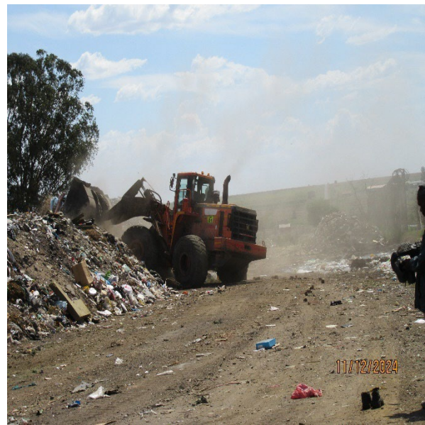
Annexure 1.23: A bulldozer was used to move waste blocking the roadway to the sides in the Sasolburg landfill site
