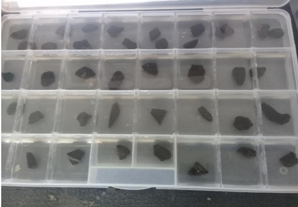
Figure 21: Chrome Slag soaked in Ethylene Glycol
