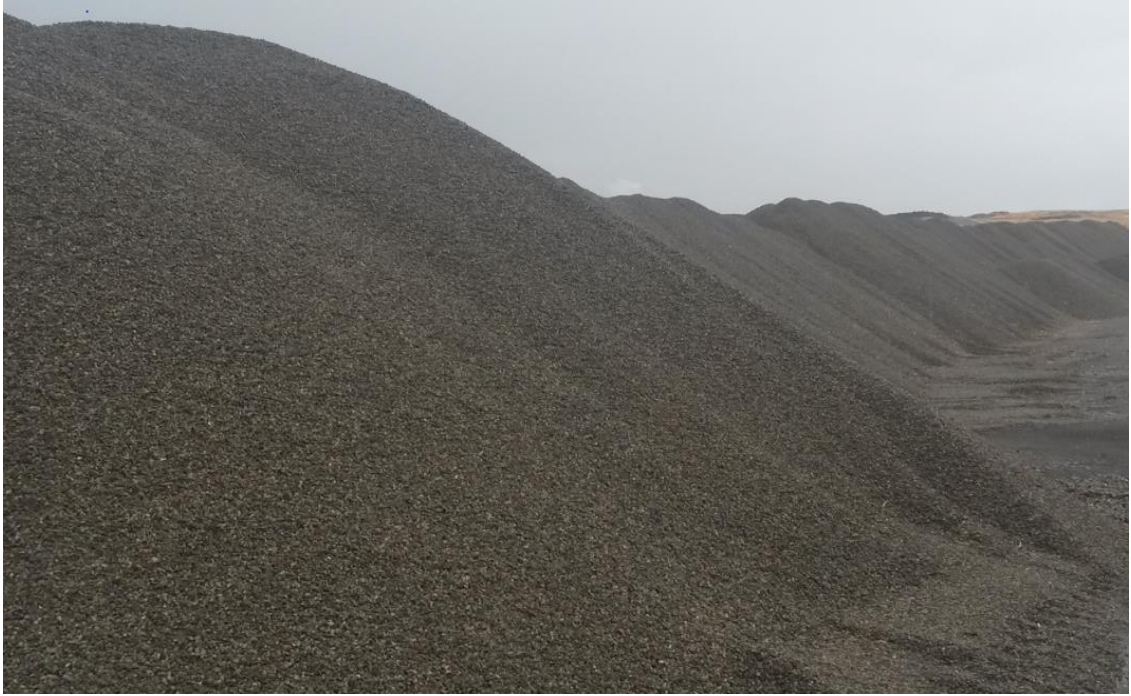
Figure 3: Processed air cool Chrome Slag
