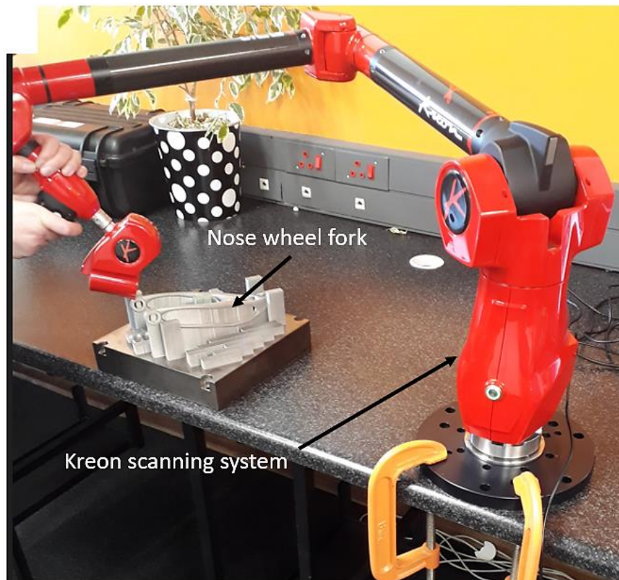
Figure 3.10: An illustration of the Kreon scanning system used to measure deviation on the L-PBF Ti6Al4V(ELI) nose wheel fork during Scan A
