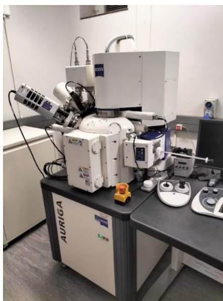
Figure 3.2: A SEM used to analyse the surface morphology of the samples.
