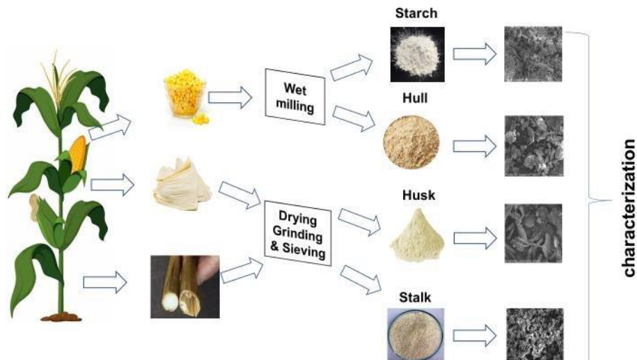
Figure 2.8: Preparation and extraction of corn biomass (Ibrahim et al., 2019).
