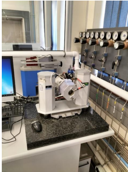
Figure 3.4: Perkin-Elmer DMA utilized to determine dynamic mechanical properties of samples.
