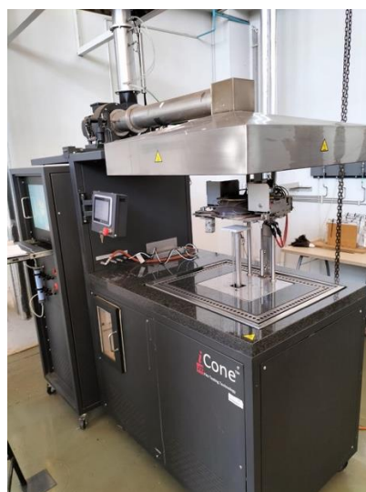
Figure 3.5: A cone calorimeter used to analysis the flammability of the samples.
