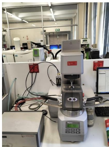
Figure 3.6: The rheological properties of the samples were studied using a rheometer.
