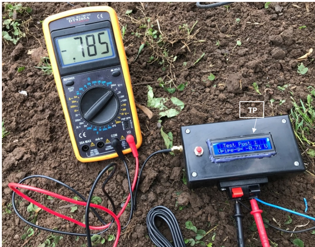
Figure 5.7: Ground test with reference to CSE
