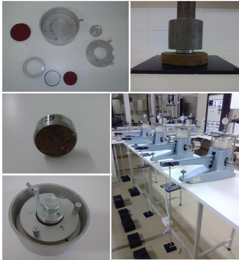
Figure 5.16: Swelling stress test setup
