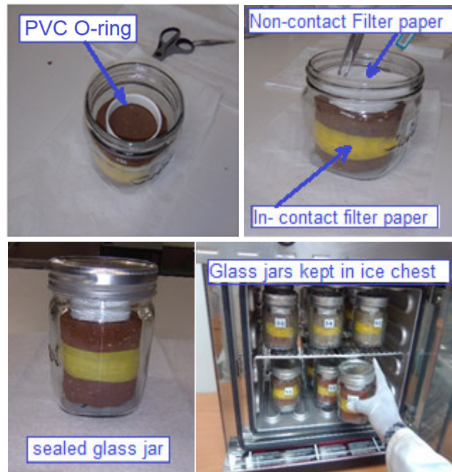
Figure 5.13: Non-contact and in-contact filter paper for total and matric suction measurement
