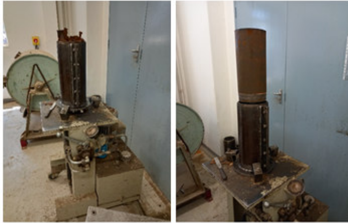
Figure 5.18: Specimen extruder setup
