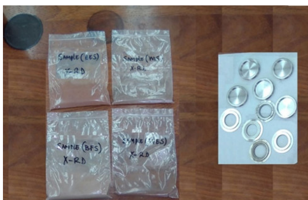
Figure 5.3: Samples preparation by front loading for XRD test
