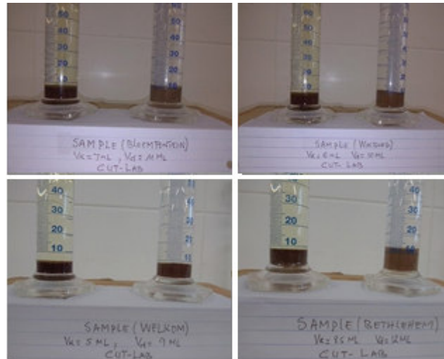
Figure 5.5: Free swelling index test setup
