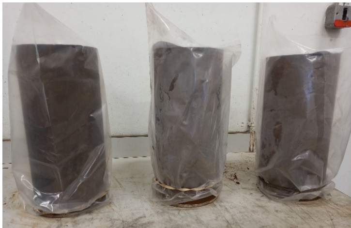
Figure 5.19: Specimens awaiting triaxial testing
