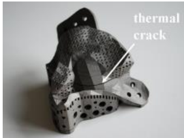
Figure 15: L-PBF part with crack induced by thermal stresses (Kruth et al., 2012)
