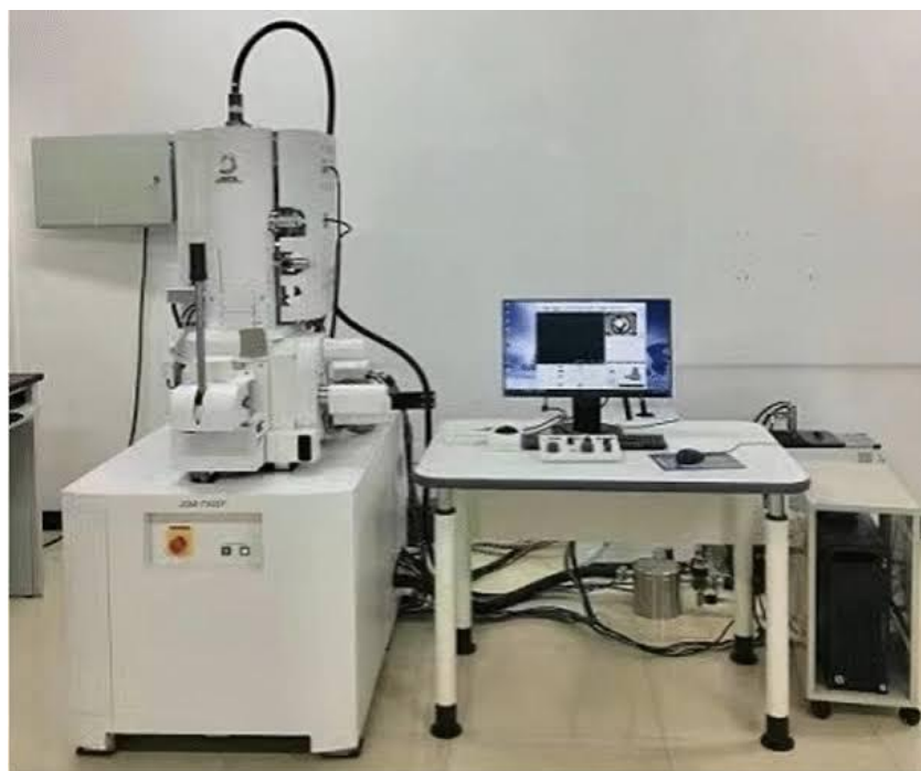
Figure 3.3. JEOL JSM-7800F Extreme-resolution analytical field emission scanning electron microscopy. Source: Fan et al. (2023)
