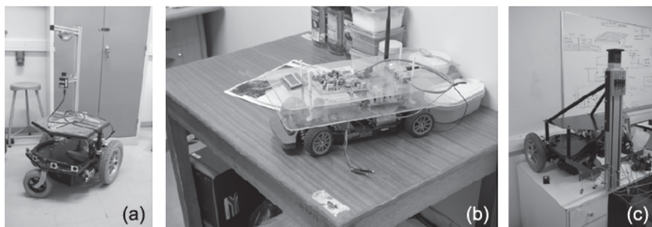
Figure 1: (a) An AGV with 360 view camera for RGEMS. (b) A small AGV using GPS for RGEMS. (c) Newly constructed AGV with Robot gripper to be installed in the front for RGEMS.
