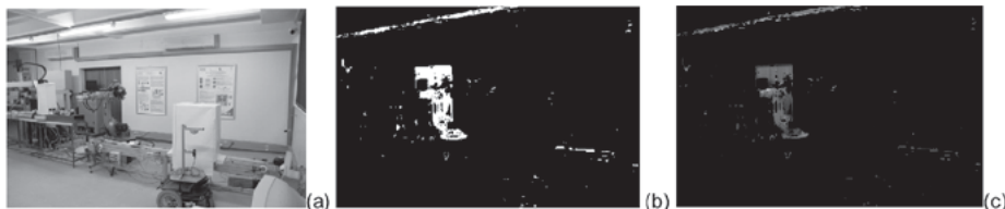
Figure 6: (a) A colour image of the automated workplace. (b) Example of the automated work place with the hue filter of a window from 6.16 radians to 6.406 radians (orange range). (c) The colour image of (a) masked with (b) showing the orange KUKA robot and orange electricity channel in roof.
