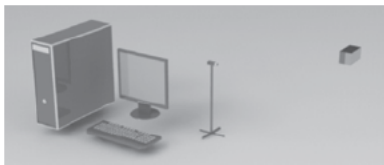
Figure 3: Concept of the stationary camera and hardware interface with the two colour object in view as drawn in Computer Added Design CAD
