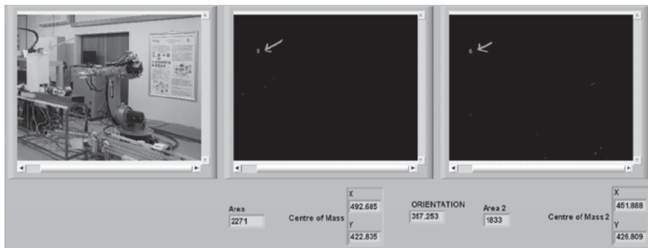
Figure 14: Screen shots of the implementation, where the object is placed in the automated work place
