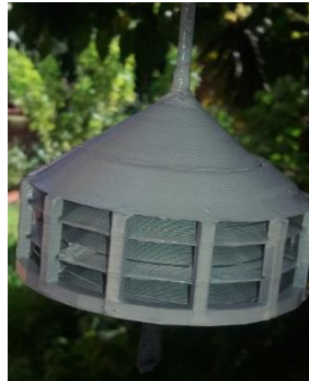
Figure 3.15: Example of the 3D-printed sensor radiant shield.
