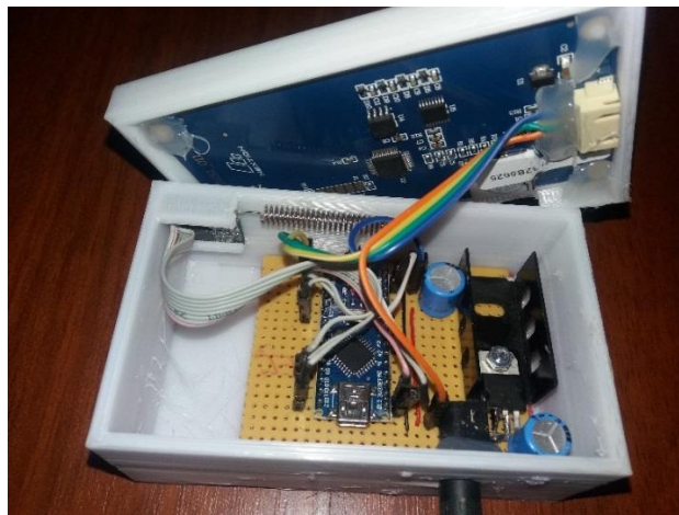
Figure B3: A 3D-printed enclosure showing perfboard with Arduino Nano, RFM95 LoRa transceiver.
