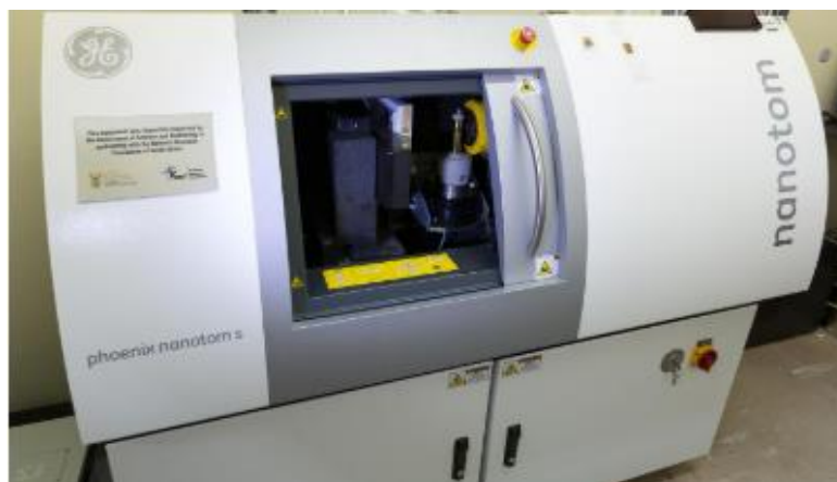
Figure 56. Phoenix Nanotom S X-Ray Tomography system installed at SU [147].
