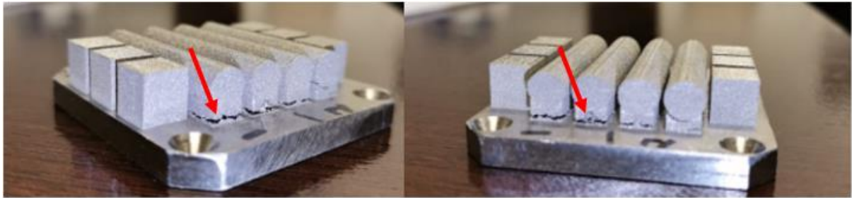
Figure 46. 3D test cubes and the failed tensile test specimens
