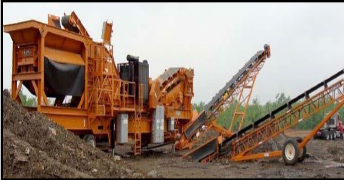
Figure 2.2: Mobile crushing plant (Texas Lone Star Materials. 2013. Available from: www.txlsm.com [Accessed 2013])
