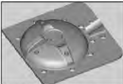
Fig. 15. Design of bottom cover core
