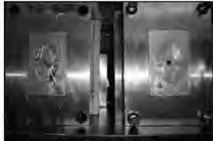
Fig.10. Cavities were machined but the small bronze insert was grown and fitted inside the mould.
