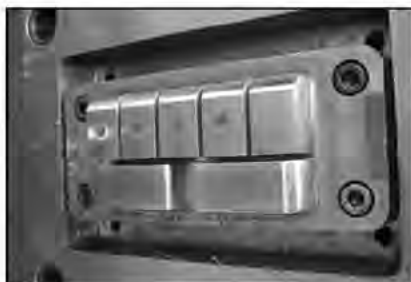
Fig. 22. Polished core with ejector pins fitted
